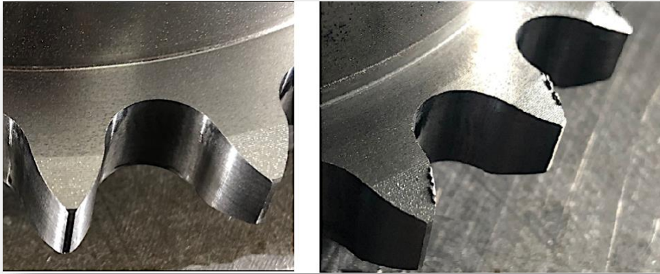
Figure 12. Visual comparison of machined tooth edges Burr-free machined part Parts machined with burrs
