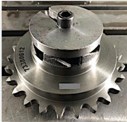
Figure 6. Ratchet attached to the machining center table
