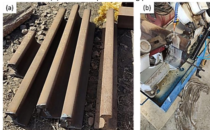
Figure 1. Preparation of rail samples for the experimental analysis, showing (a) the rails in their initial as-received condition and (b) the subsequent cutting process to create test sections
