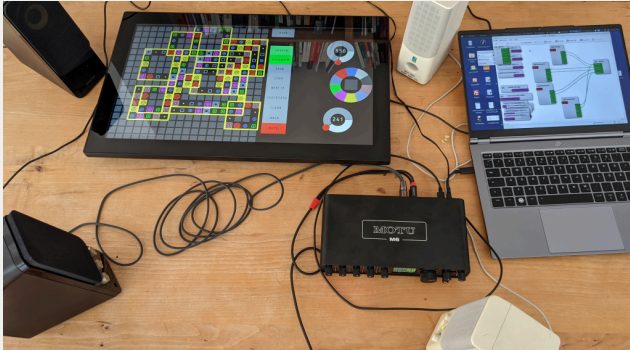
FIGURE 10. TEST SETUP WITH QUADRAPHONIC SOUND, TRANSMISSION OF MIDI DATA VIA WI-FI FROM TABLET TO LAPTOP, AND IMPROVED SOUND QUALITY THROUGH THE USE OF PHYSICAL MODELING SOFTWARE
