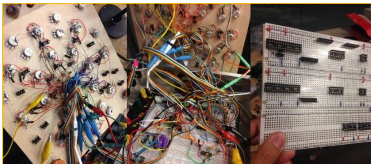
Fig. 5: Analogue Revolutions – underside of top plate (left); initial configuration on solderless breadboard (center); final layout of solderable beadboard (right).
